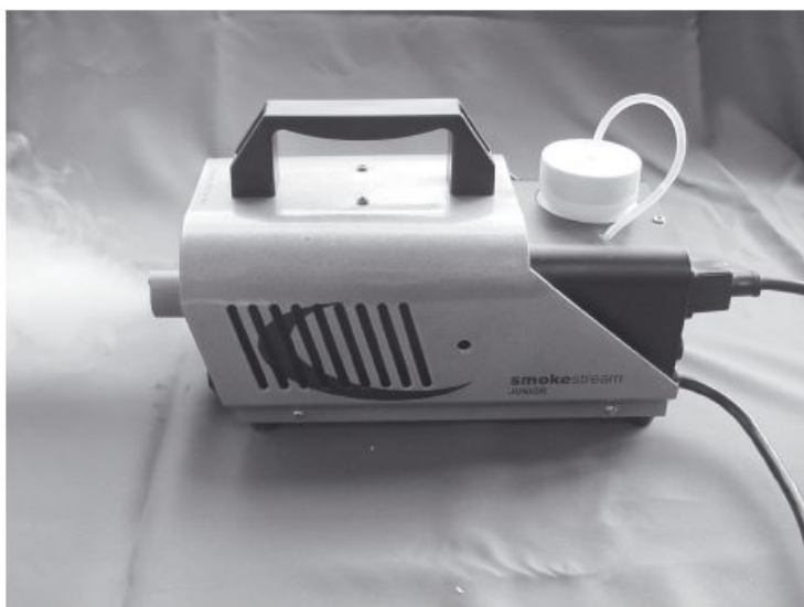
Figure 12.4 Instrument producing wisps of smoke to check air flow under door
