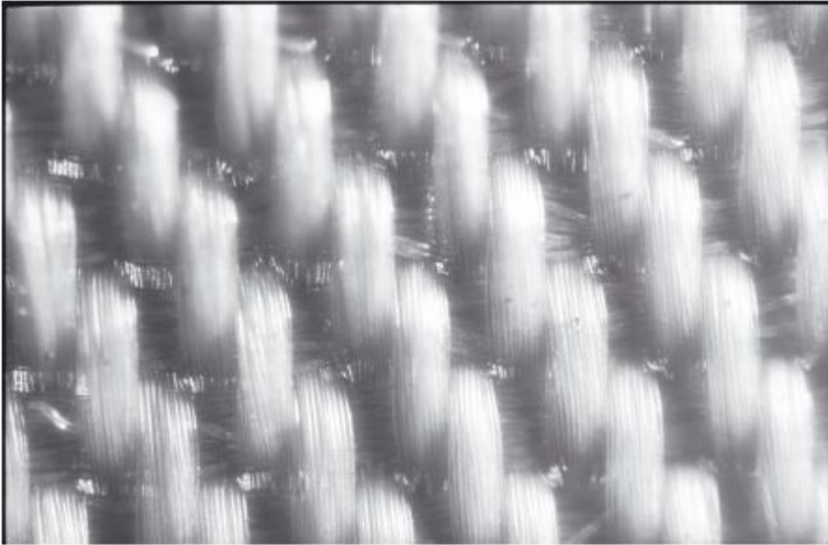
Figure 20.8 Typical construction of a cleanroom fabric
