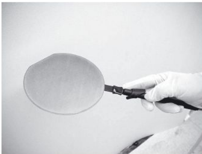
Figure 17.9 Handling with vacuum wand (good technique)
